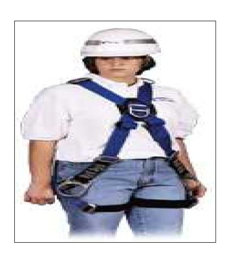
Class III- Harness that fastens around waist, around thighs or under buttocks, and over the shoulders; designed for rescue where two person loads may be encountered and inverting may occur
